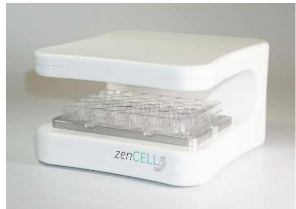
Figure 1: zenCELL owl. 24-channel microscope with 24-well cell culture plate.
