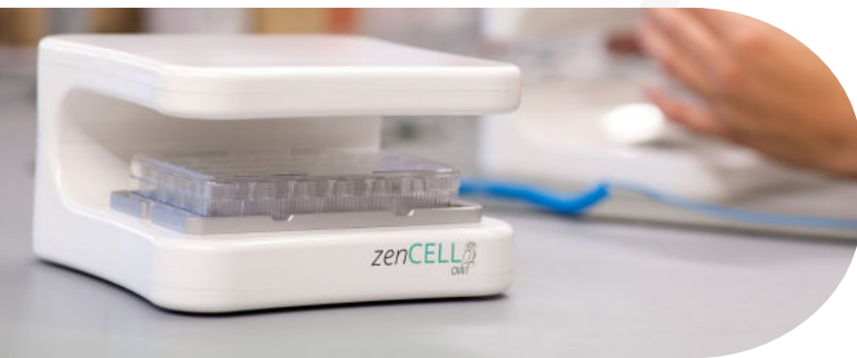
Figure 1: zenCELL owl. 24-channel microscope with magnetic adapter frame for 24-well cell culture plate.
